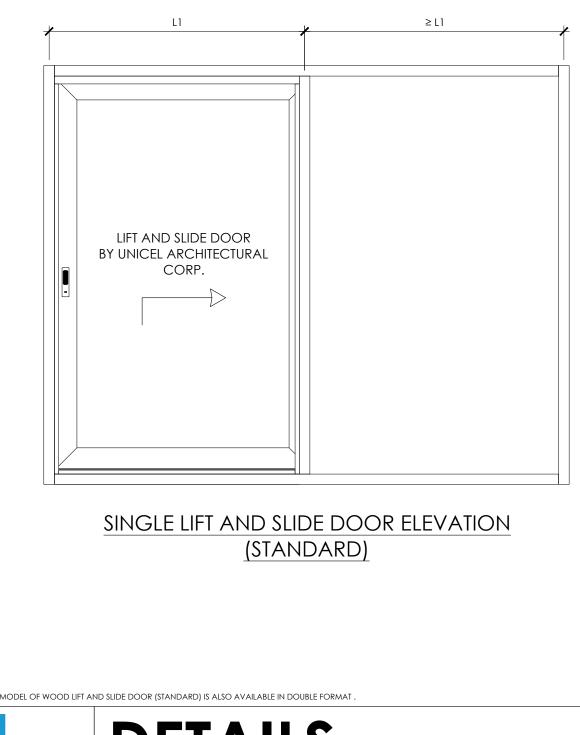
NOTE: THE MODEL OF WOOD LIFT AND SLIDE DOOR (STANDARD) IS ALSO AVAILABLE IN DOUBLE FORMAT .
