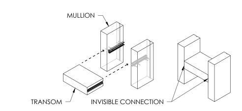
DIAGRAM 1: CONVENTIONAL TRANSOM INSERTION FROM THE INSIDE OF THE BUILDING TO THE OUTSIDE, WITH INVISIBLE MACHINING.
